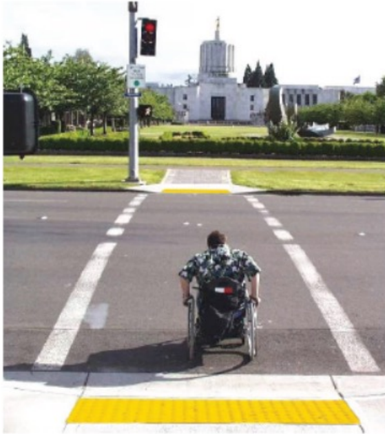
An LPI allows a pedestrian to establish presence in the crosswalk before vehicles are given a green indication.
