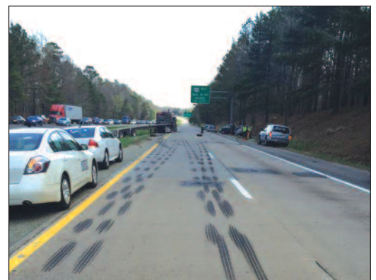
Fig. 10—Appearance of locked wheel skip skid marks made by an empty trailer.
