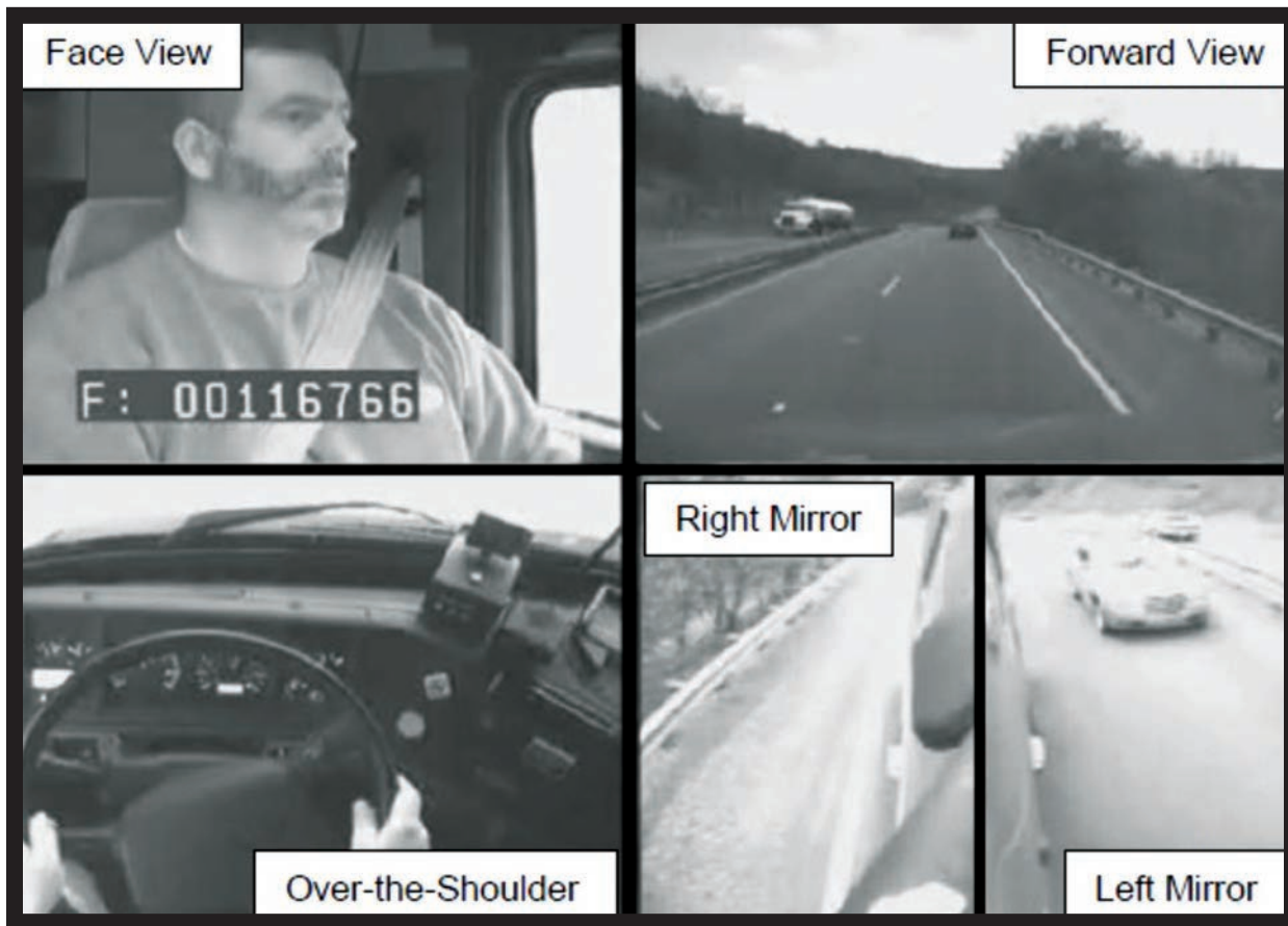
Figure 2 —Split-screen presentation of the five camera views used in a naturalistic truck driving study.
