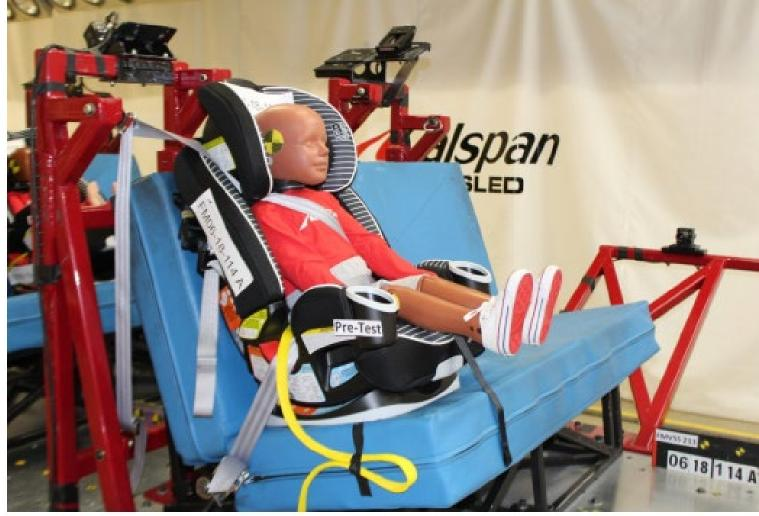
• Other FMVSS No. 213 requirements include webbing strength, durability, material flammability, buckle release before and after the test, labeling, compatibility with attaching to the vehicle's child restraint
