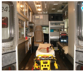
Prior to crash equipment and gurney either mounted or stowed in cabinets
