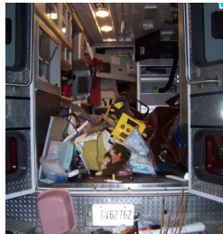
Post crash (rollover) equipment and gurney positions drastically changed
