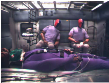
Frontal Crash: 30 mph into a rigid wall This is the same test used in passenger vehicles
